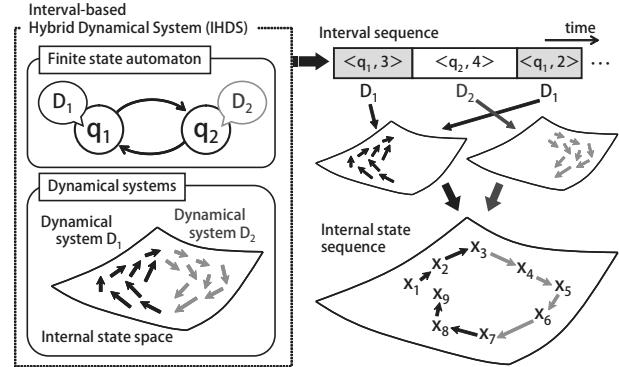
Figure 2. Interval-based Hybrid Dynamical System (IHDS).
