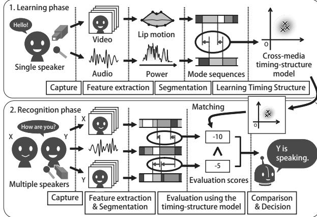
Figure 1. Flow of speaker detection using the timing structure.
