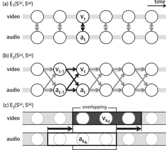
Figure 10. Temporal relations used in each of the evaluation functions. (a) Mode pair co-occurrence in the same frame. (b) Mode transition probability between the adjacent frames. (c) Temporal difference of overlapping interval pairs (proposed method).
