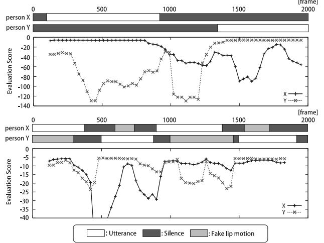
Figure 11. Examples of temporal change in the evaluation scores. The top part of each graph shows the state of lip motion. The upper graph is the case that no fake lip motion occurs, and the lower one is the case that fake lip motion is included in most frames.
