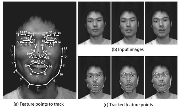
Figure 6. Examples of (a) a training image to build AAMs, (b) a captured face images, and (c) face images with tracked feature points.
