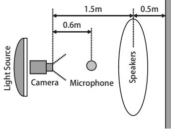
Figure 4. The layout of the recording room
